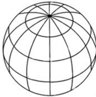
Figure 5. Convergence of longitude lines produces shrinking 1^\circ \times 1^\circ rectangular grid cells toward the poles.
