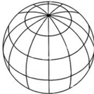
Figure 3. Convergence of longitude lines produces shrinking 1^\circ \times 1^\circ rectangular grid cells toward the poles.
